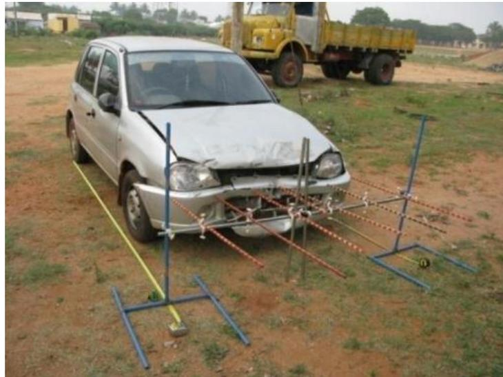
Figure 4. Crush Profiling
